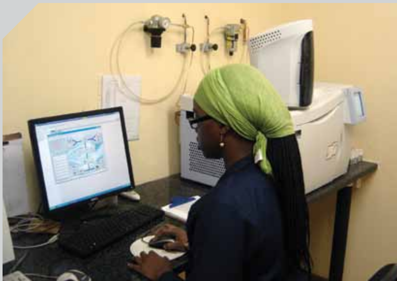
The use of the Gas Chromatograph (GC) for the determination of fuel dilution in engine oils is a particularly involved analysis that requires skilled lab technicians. Here, lab assistant Nozipho Ngubane operates WearCheck's new Perkin Elmer GC Clarus 580 in the Middelburg laboratory
