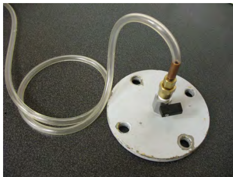
Ensure that the sampling hose valve and flange is clean on the inside and outside.
