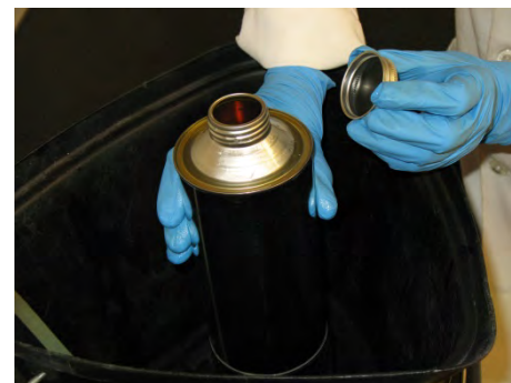
Squeeze the sampling tin until the oil overflows. Fit the lid (with nitrile rubber seal) to the tin whilst oil is overflowing.
