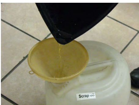
Discard oil from the sampling bucket into a scrap oil container.
