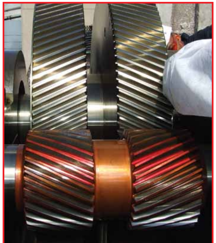
Figure 1: Varnish on centrifugal compressor gears [picture courtesy Higrotek]
