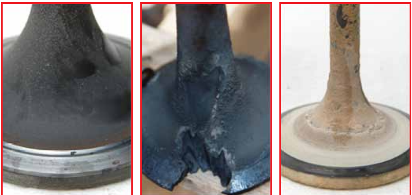
From left to right pictures of a good valve, a torched valve and a recessed valve courtesy of Infinium International Limited
