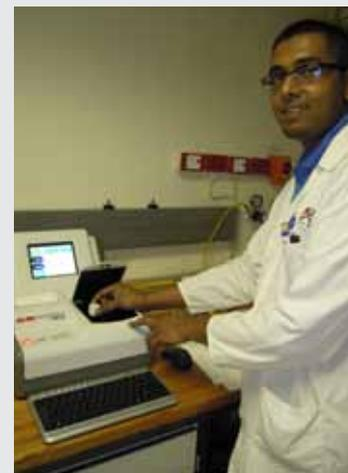
*WearCheck laboratory supervisor Shiven Brijlal uses one of their two new X-ray fluorescence spectrometer (XRF) analysers to test for the elements sulphur and chlorine content in fuel and oil samples. The new XRFs, which are installed in WearCheck's fuels laboratories in Gauteng with one to follow in Zambia, have boosted service delivery by yielding highly accurate results in record time*
