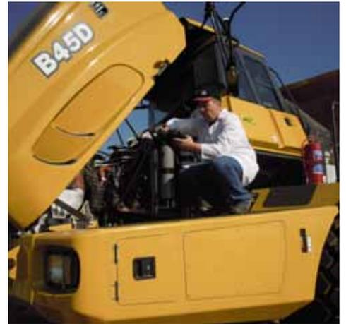
*Employing the latest specialist vibration and thermographic testing techniques, WearCheck's new reliability solutions division works to ensure that machinery reaches its projected life expectancy and beyond, where possible; and to increase the reliability of plant. Here, vibration and oil technician Marcelle Symons takes a vibration reading from a Bell B45D dump truck enrolled in the new programme*
