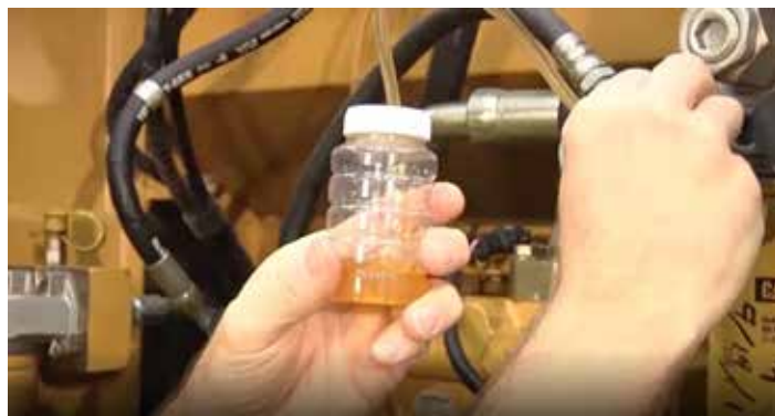
An efficient filtration system helps to enhance the useful life of oil, which should be regularly sampled and monitored
