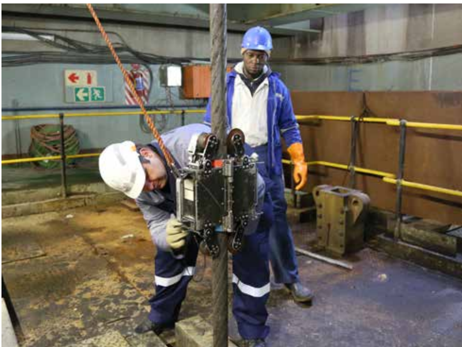
WearCheck technician Roger Henwood (a SAQCC RCA level 2 senior rope inspector) uses a magnetic rope test instrument to test the integrity of steel wire rope. Looking on is rigger assistant from the mine
