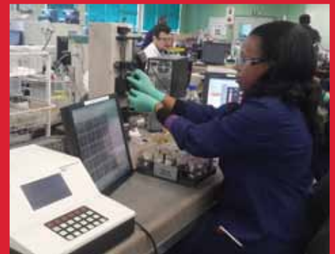
A lab technician operates one of WearCheck's particle counters, which measures the cleanliness of diesel samples as per ISO 4406
