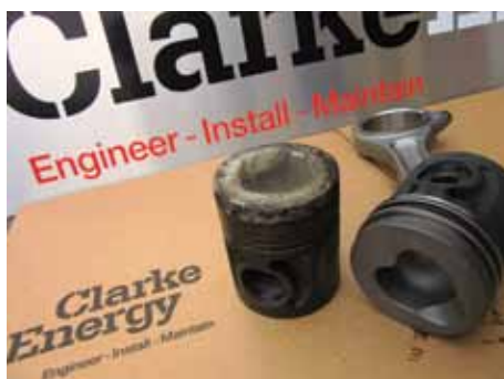
Image of a new and siloxane coated piston courtesy of Clarke Energy
